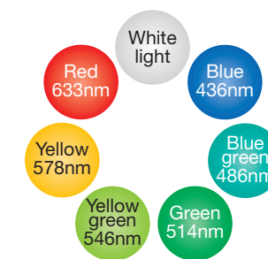
Multi layer observation using wavelength selection (concept illustration)
