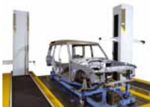
LK H-R dual column horizontal arm CMM
