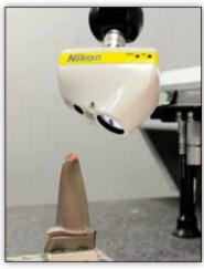
Turbine blades Eliminate probe tip compensation
